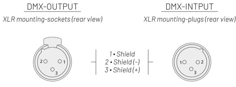
When using standard DMX512 control signal, the last device's output interface must be connected to a DMX plug. This plug is putting a 120 ohm resistance between "canon" plug's 2 pin and 3 pin. Showing as below pic. Sticking this plug into the last device's signal output interface, it will avoid the interference during the process of signal transmission.
